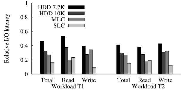
Figure 9: Relative I/O Latencies for Different Write Caches.
